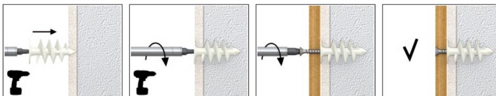
1. Drive R-ISO-PLUG into the insulation material (manually, or with an electric screwdriver) until installation depth reached.
